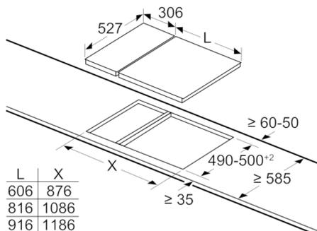
When installing a Domino unit right next to a hob, an assembly kit (HEZ394301) is required.
